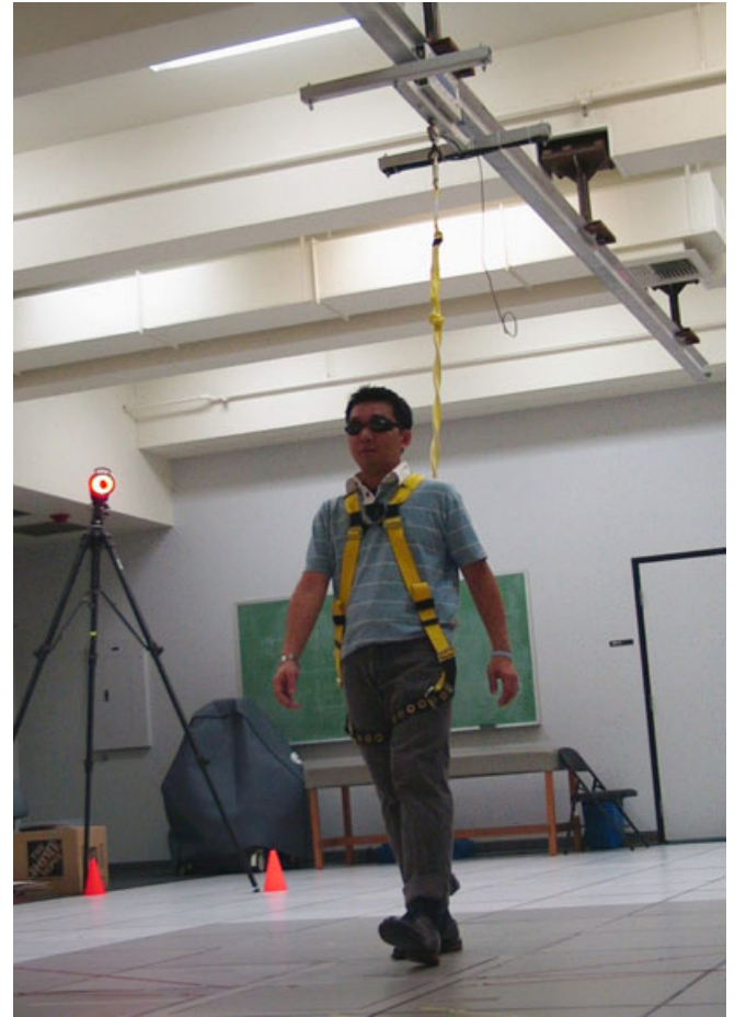
FIG. 2—During all walking trials, subject wore a fall-arresting safety harness attached via a nonstretch lanyard to an overhead trolley.
